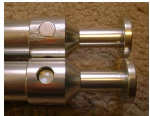
Figure F. Two aluminum bolt examples: the top bolt showing the Neodymium magnet installed and the bottom bolt showing the hole where the upper surface of the steel bolt pin is visible.
