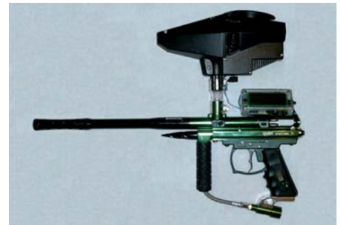
Figure E. The marker with the electric loader on top and the ShotMeter mounted on the sight rail between the grip and the loader.
