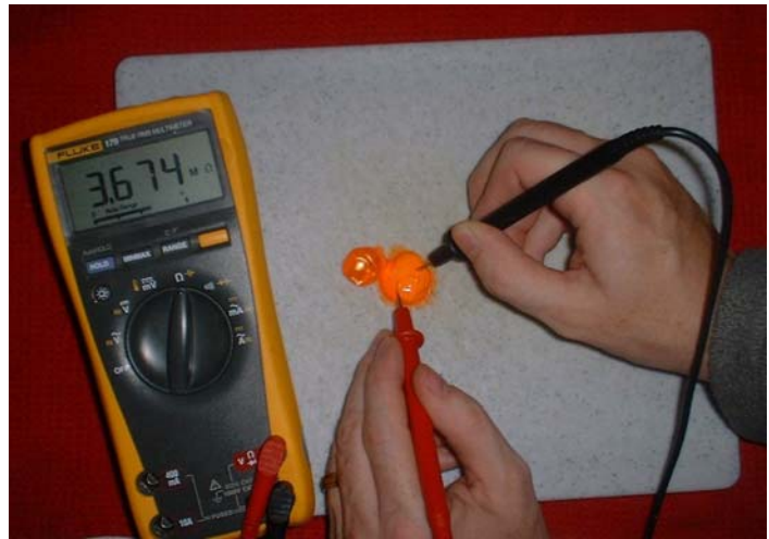
Figure C. Measuring the resistance of a glob of paint.
